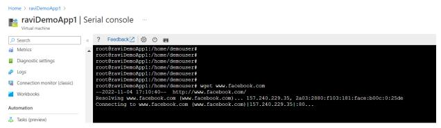
Connection won't be established. Go to **Azure Log Analytics** to validate that Cloud NGFW has blocked this connection as per the rRulestack configuration.
